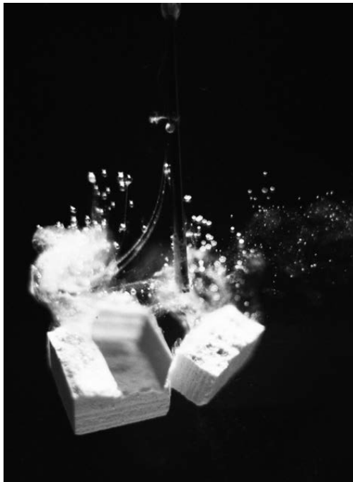
Fig. 7: Effect of a focused shock wave on an artificial stone
